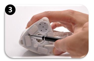
Next, one has to push the button with a locked padlock symbol once again and hold it until the yellow diode turns off. Turning off of the yellow diode indicates that another USER remote control has been programmed.
