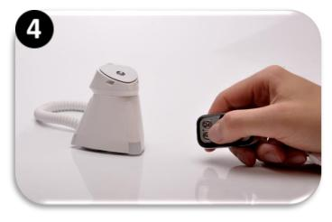
After programming the USER remote control one has to assemble the anti-theft system and make sure whether its operation is correct. Aim a USER remote control at the armed V-line and push the button with an unlocked padlock symbol. The V-line should then disarm.
